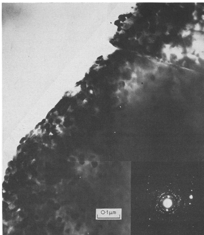
Figure 1 Electron transmission micrograph showing Te precipitation together with diffraction pattern (inset).
